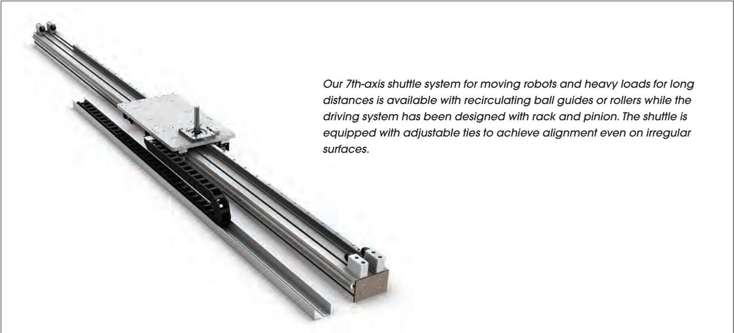
*Our 7th-axis shuttle system for moving robots and heavy loads for long distances is available with recirculating ball guides or rollers while the driving system has been designed with rack and pinion. The shuttle is equipped with adjustable ties to achieve alignment even on irregular surfaces.*
